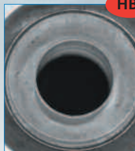
Kel-F valve seats in HBr Service, with NANOCHEM® purifier, 1000 cycles.
