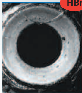
Kel-F valve seats in HBr Service, without NANOCHEM® purifier, 1000 cycles.
